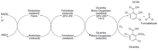
Figure 4: Components of the dicamba O-demethylase system
